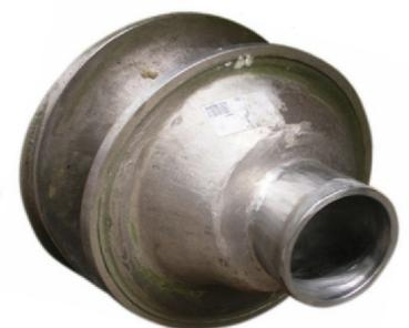
A typical F-type impeller
